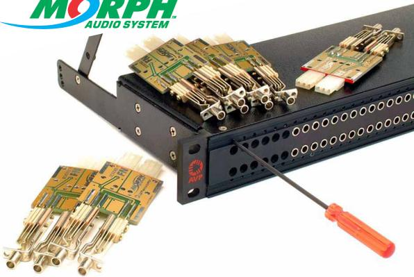
Keep an inventory of Morph Modules and empty Morph frames to allow custom jackfield assembly or re-configuration in minutes! Morph modules fit 1, 1.5 & 2 Rack Unit frames.
